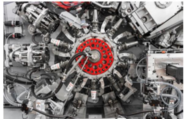
The centerpiece of the machine is the cup-shaped unit or “star.” This unit has a diameter of approximately 1 m and is equipped with core spikes. The unit must be accel-
