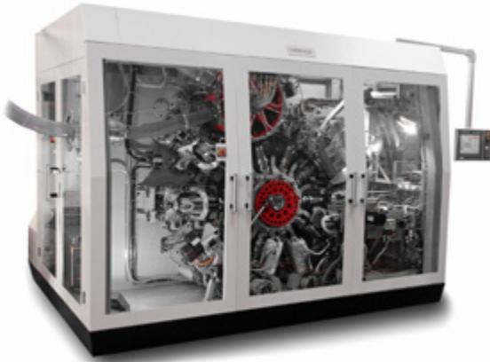
Firstly, voltage surges put a heavy strain on the drives and thus led to failures. Secondly, the regenerative energy was converted into heat during braking, as a result of which the braking resistor temperatures rose to 80°C. Due to the use of highly flammable paper, it was not possible to install the braking resistors outside the control cabinets. The excess heat therefore had to be discharged from the control cabinets at a significant cost.
