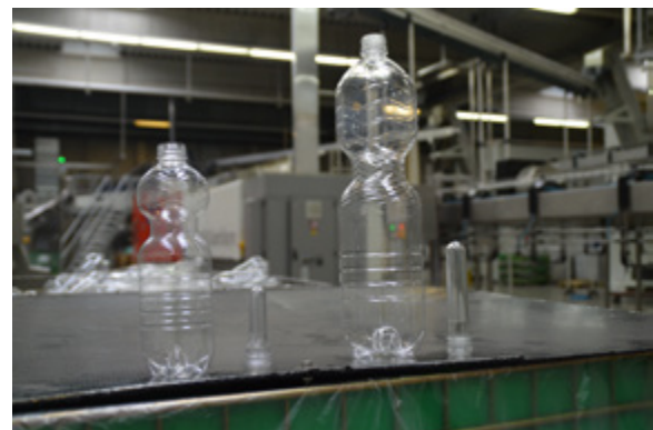
The familiar PET bottles are generated from these preforms in the blowing hall.
